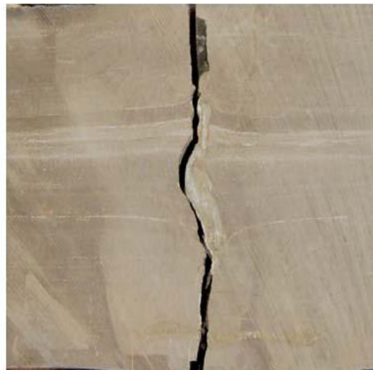
Figure 4 - Small, Early, Compacted Veins, Fill Likely Dolomite; and (picture to right) Example from New Albany Shale Core at 2,804 ft. Height of Fractures Approximately 3 cm. Reference 3.
