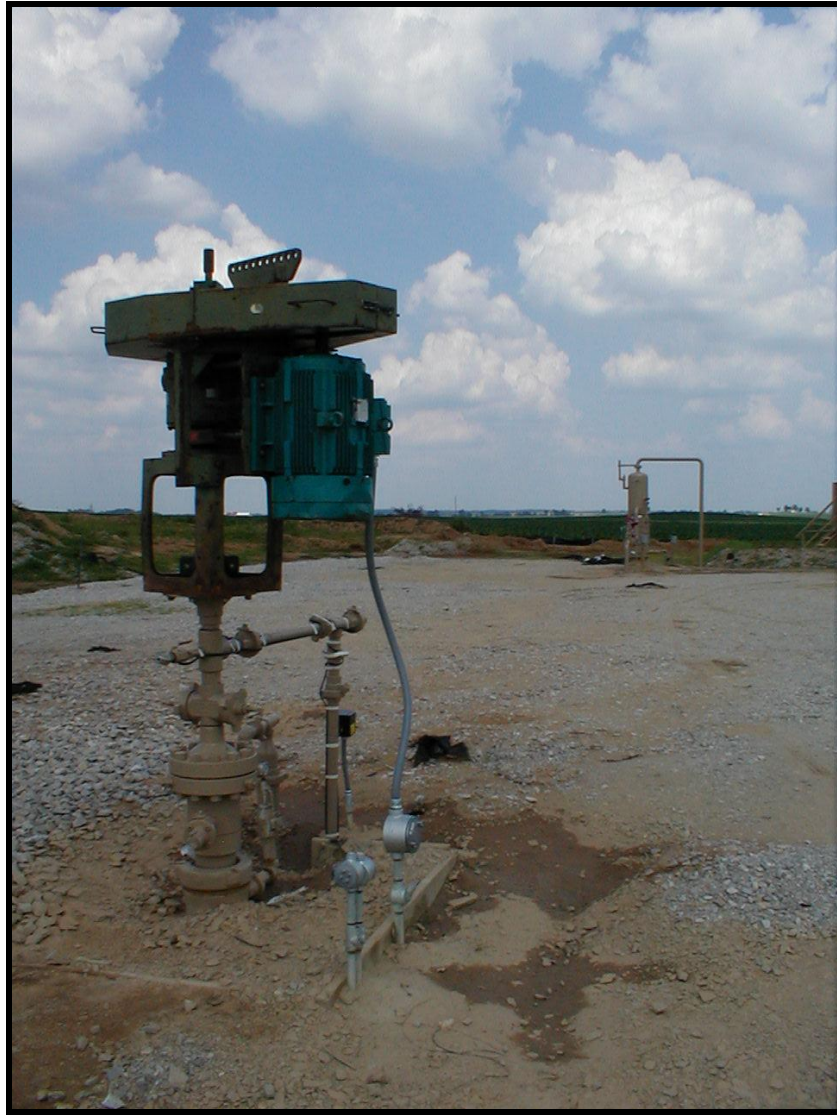
Figure 7–Surface Configuration for Progressive Cavity Pump – From Aurora Oil and Gas 4
