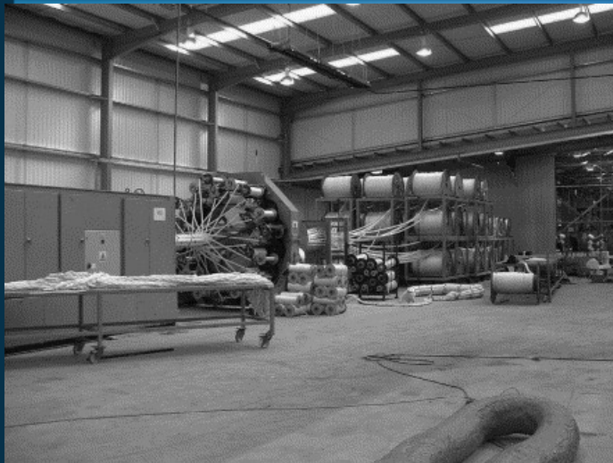
Rope Braiding Machine fabricating Mooring Line
