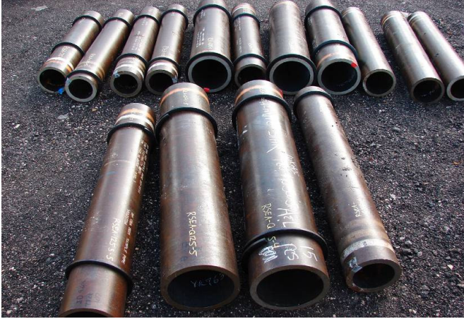
FIGURE 3: TEST PIPES WITH OUTER DIAMETERS RANGING FROM 284 mm TO 406 mm AND WALL THICKNESS FROM 14 mm TO 34 mm.
