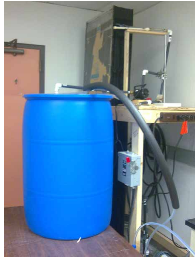
Steam to heat inlet batch feed
