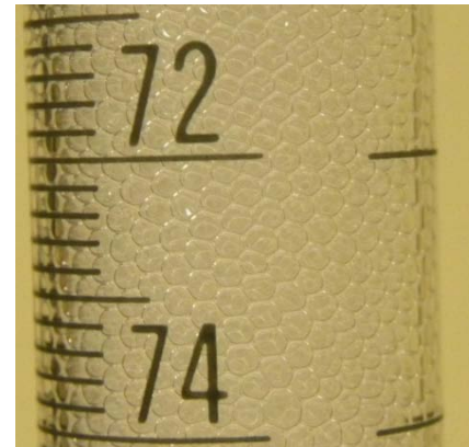
Bubble size: 1 mm (low flow rate)
