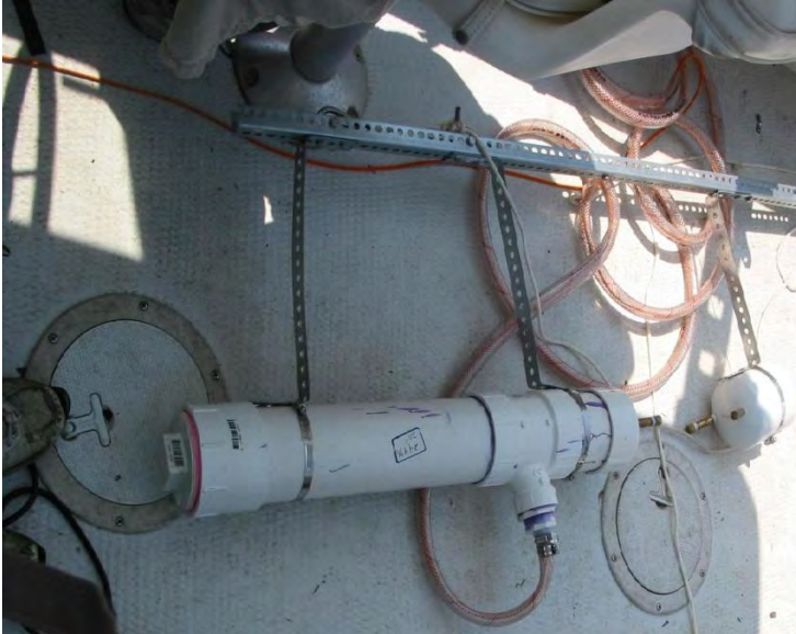
Figure 3 Picture of the frame holding the transmitter (right) and the receiver (left) containers.
