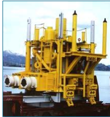
Draugen, worlds 1st commercial subsea multiphase pump installed
