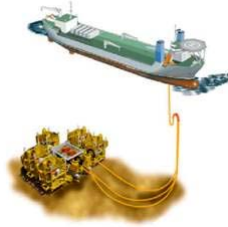
Draugen, worlds 1st commercial subsea multiphase pump installed
