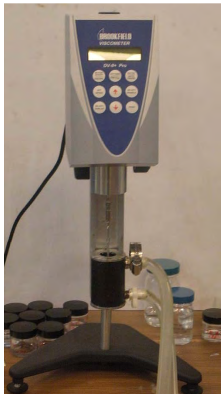
Photographs of (a) Brookfield DV-II +Pro, and (b) DV-I prime digital viscometers from the PEER Institute laboratory.
